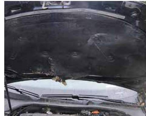
Damaged insulating matting
