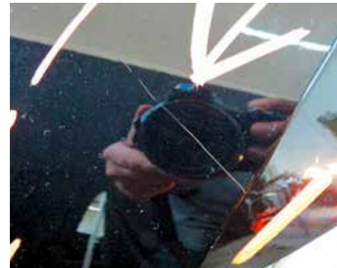
Damage to base paint
