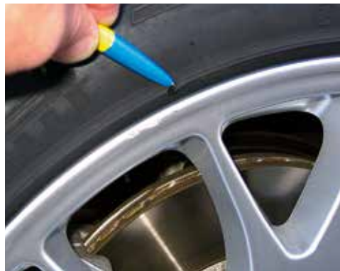
Minor material loss on the wear strip
