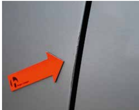
Minor paint damage on door edges
