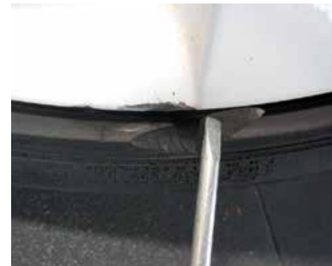
Tyre wall damaged
