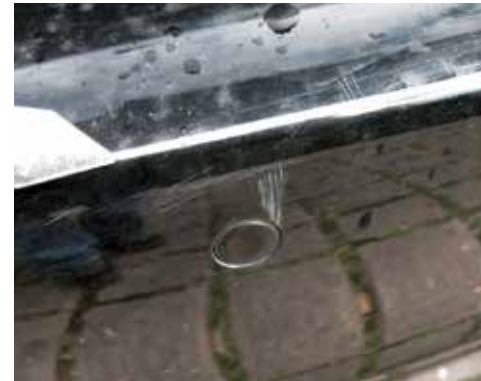
Paint damage on the bumper
