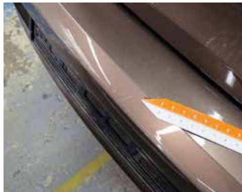
Minor paint abrasion
