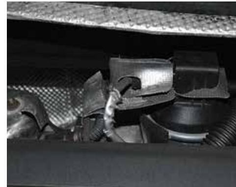
Damage due to rodents
