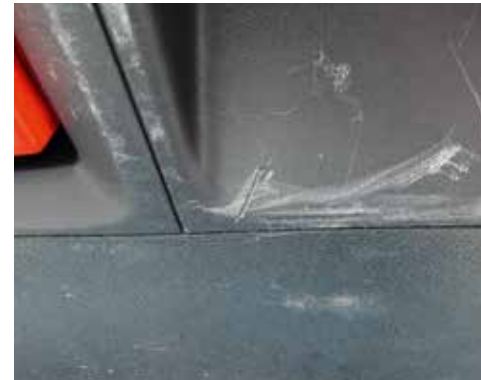
Severe scratches and scuffing
